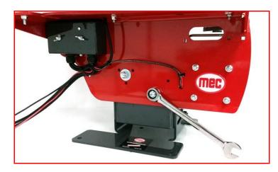
**Step 9** – Adjust the machines tilt by loosening the  $\frac{3}{4}$ " nut on the front and rear on the base of the machine, as shown below. Tilt the machine to the desired angle and then retighten both nuts securely.
